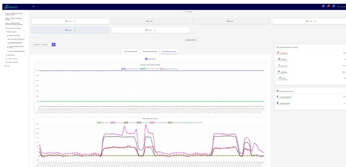
Figure 3-17: Monitoring System user interface showing real-time indoor and outdoor measurements alongside energy consumption and power factor time-series, enabling detailed analysis of building performance
