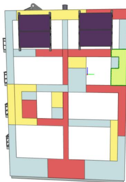
Figure 23 Close-up of the BIPV panel on the south-west facade of the building
