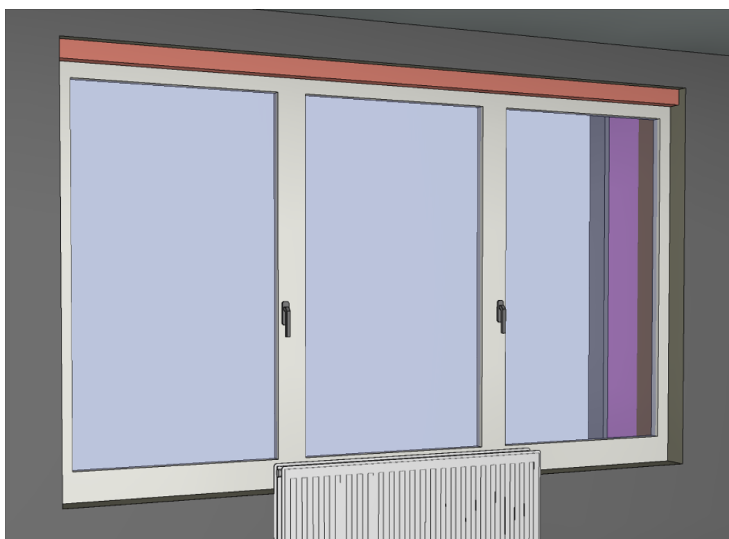
Figure 13: New windows with high-performance double glazing and roller shutters
