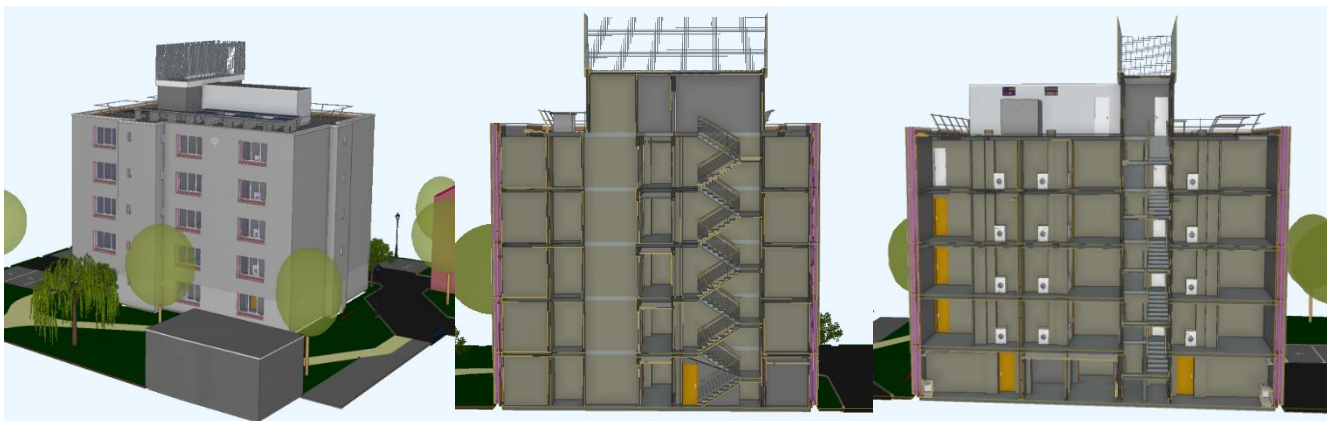
Figure 9: French BIM model post renovation – Section
