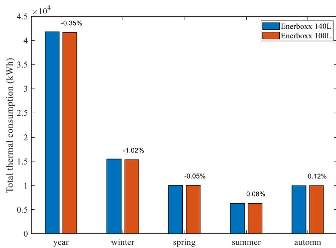
Fig. 19. Total thermal consumptions of enerboxx scenario with 140 L and 100 L tanks. (the deviations are shown in the chart).
