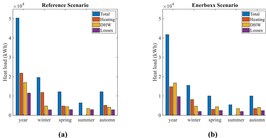
Fig. 16. Thermal consumption due to heating, DHW and thermal losses at a) reference and b) enerboxx scenarios.
