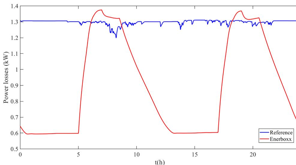
Fig. 13. Network thermal losses on a typical winter day.
