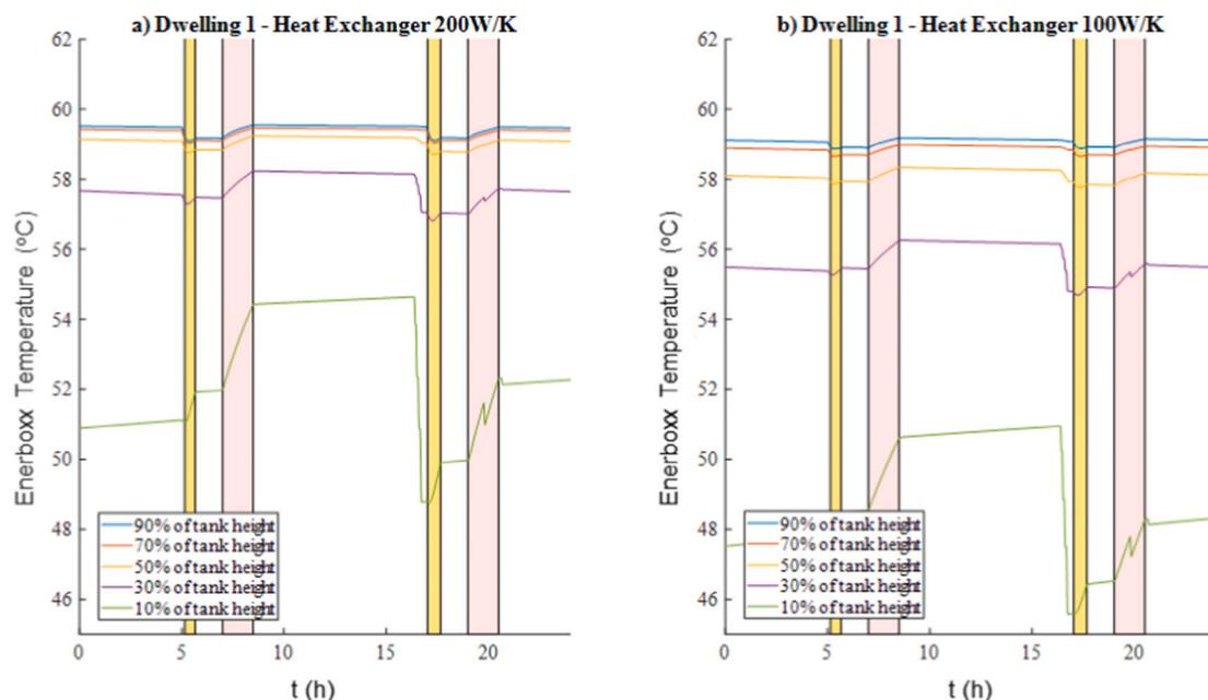
Fig. 20. Spatial distribution of water tank temperature during the time period of a typical winter day at five heights of 140 L tanks with total thermal transmittance of the tank’s heat exchanger at a) 200 W/K and b) 100 W/K.
