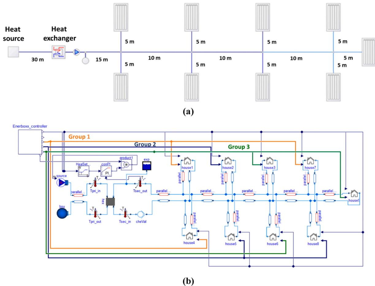
Fig. 6. Developed model of the enerboxx scenario a) in the schematic diagram and b) in the INTEMA including heat exchanger, decentralized storage tanks, piping network and dwellings (see Appendix A for the detailed explanation of the components).
