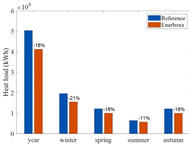
Fig. 17. Total thermal consumptions of enerboxx scenario compared to the reference. (the deviations are shown in the chart).
