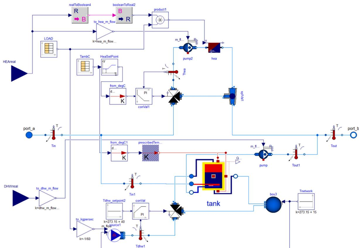
Fig. 7. Model of a single dwelling for the enerboxx scenario in the INTEMA, including key components controllers for the heating circuit and the DHW circuit (see Appendix A for the detailed explanation of the components).
