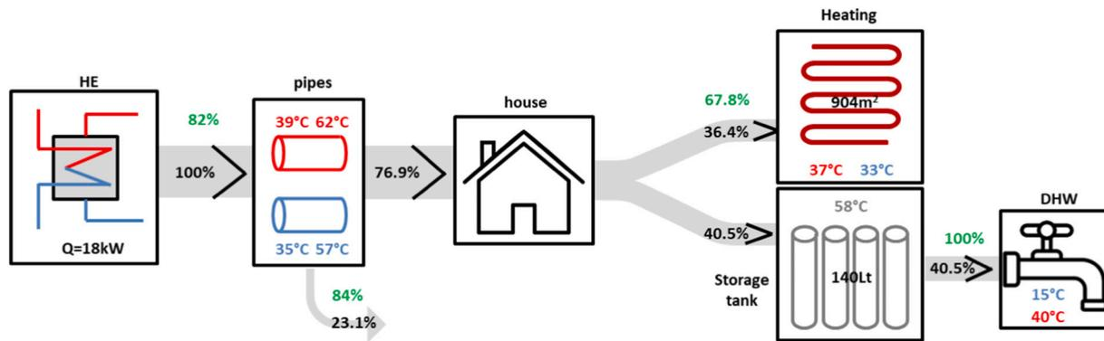
Fig. 15. Sankey diagram of enerboxx scenario for the dwelling (with green values are depicted the thermal consumptions in relation to the corresponding ones of the reference scenario). (For interpretation of the references to color in this figure legend, the reader is referred to the web version of this article.)
