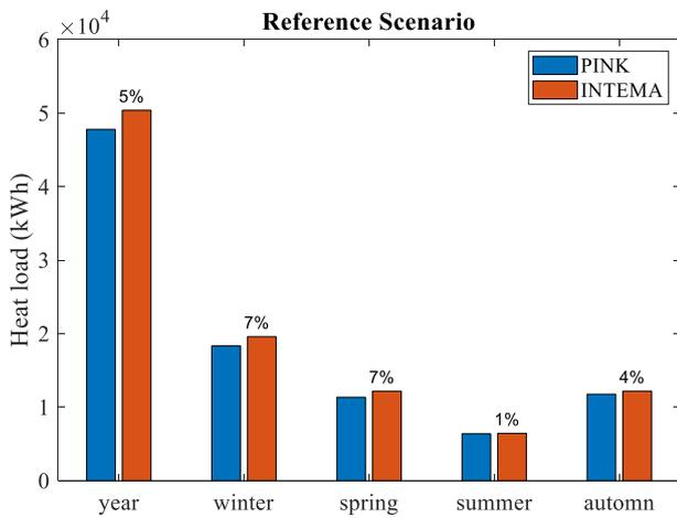
Fig. 11. Comparison of INTEMA and PINK models' annual total heat load at reference scenario (the deviations between INTEMA to PINK consumption are displayed in the chart).
