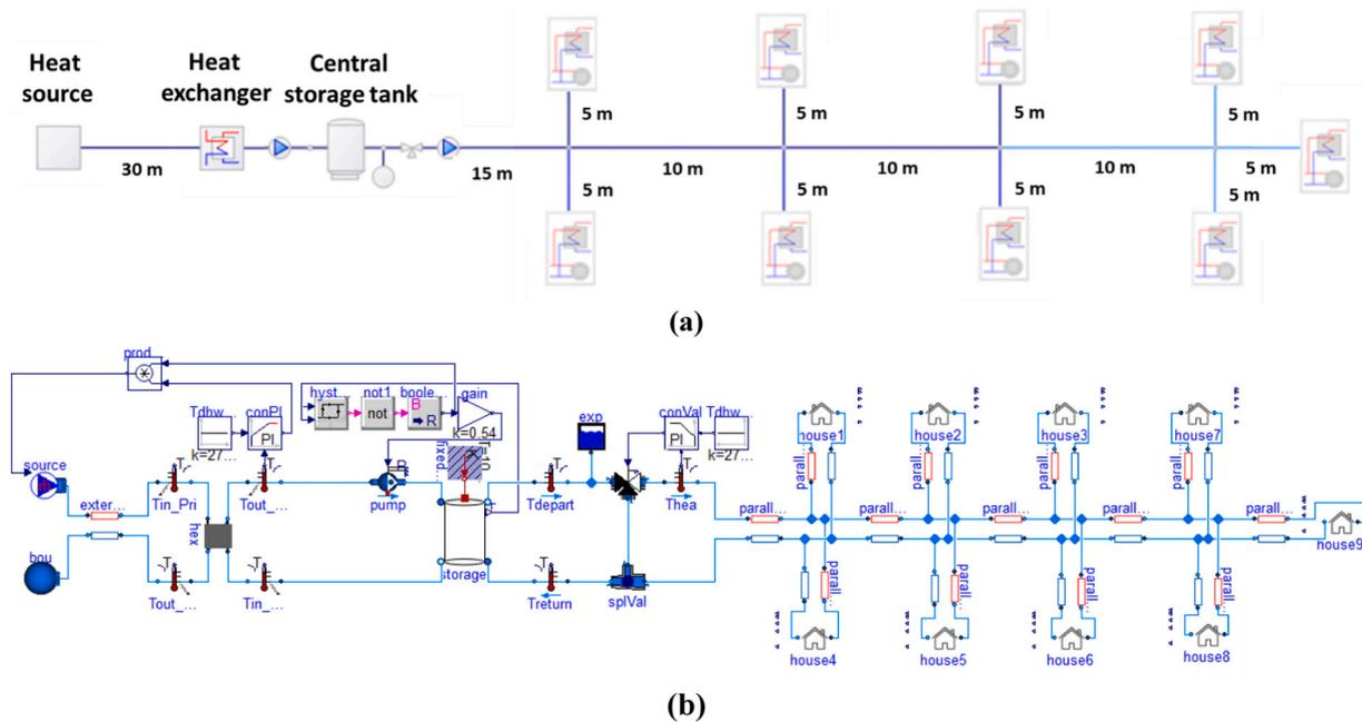
Fig. 4. The developed model of the reference scenario a) in the schematic diagram and b) in the INTEMA, depicting each of the key components with their controllers, accounted for heat exchanger, central storage tank, piping network and dwellings (see Appendix A for the detailed explanation of the components).
