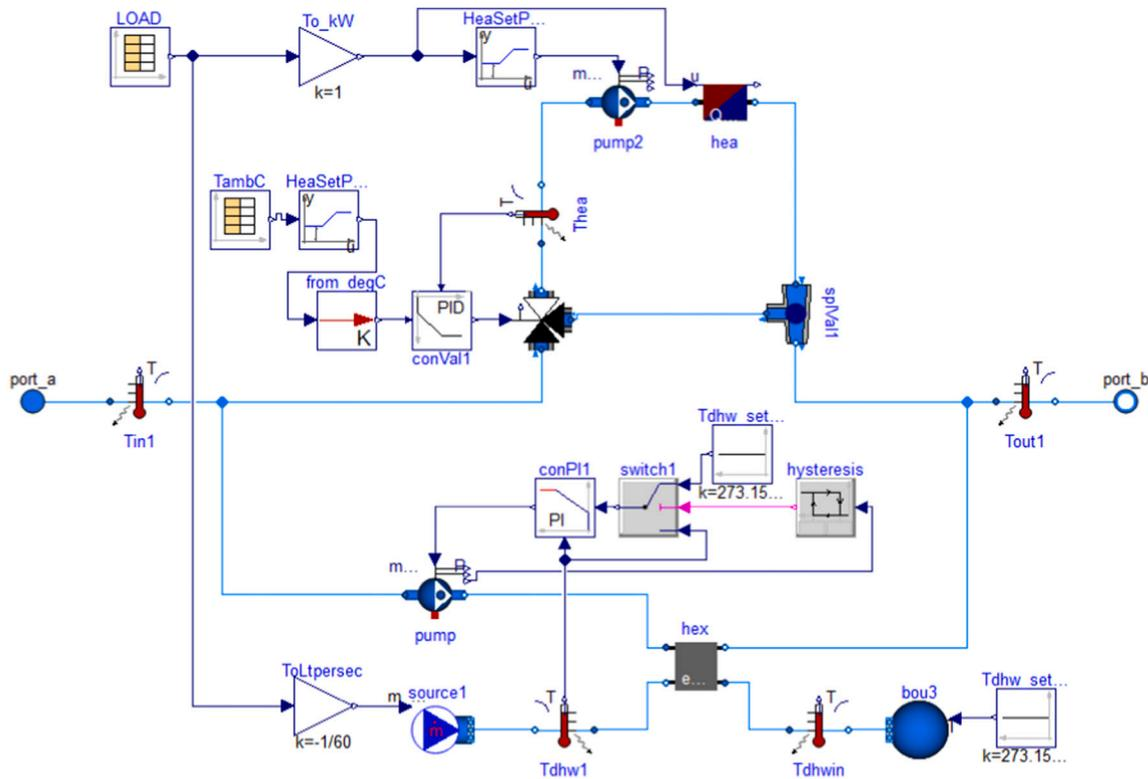
Fig. 5. Model of a single dwelling for the reference scenario in INTEMA environment, including their controllers for the heating circuit and the DHW circuit (see Appendix A for the detailed explanation of the components).
