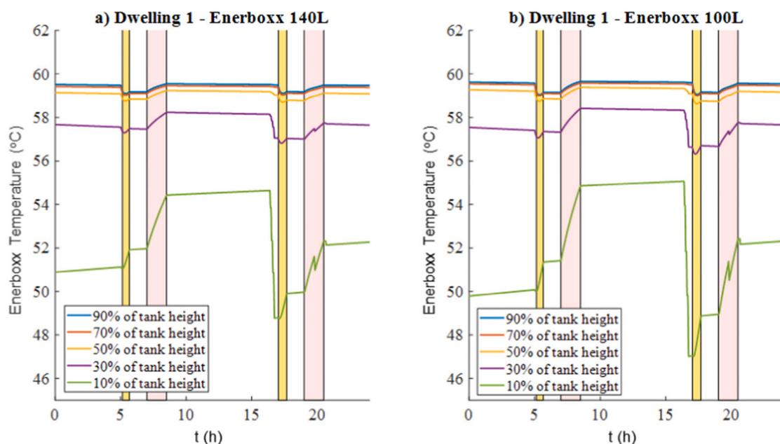
Fig. 18. Spatial distribution of water tank temperature during the time period of a typical winter day at five heights of a) 140 L enerboxx and b) 100 L enerboxx, with 200 W/K total thermal transmittance of the tank's heat exchanger.
