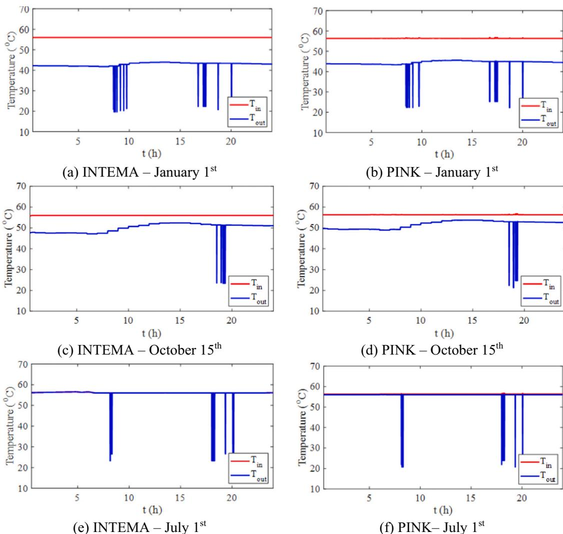
Fig. 9. Dwelling 1: Comparison of the INTEMA results with the PINK results for the reference scenario on different typical days during the year.
