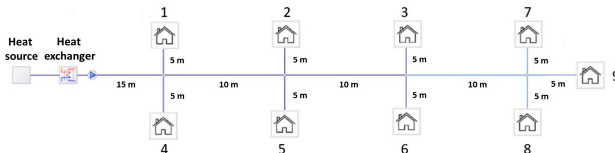
**Fig. 1.** District heating network topology under examination with piping details.
