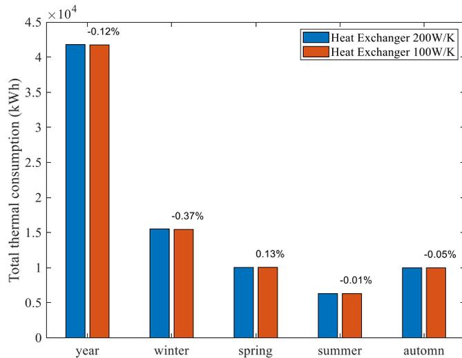
Fig. 21. Total thermal consumptions of enerboxx scenario with 200 W/K and 100 W/K total thermal transmittance of the tank’s heat exchanger. (the deviations are shown in the chart).
