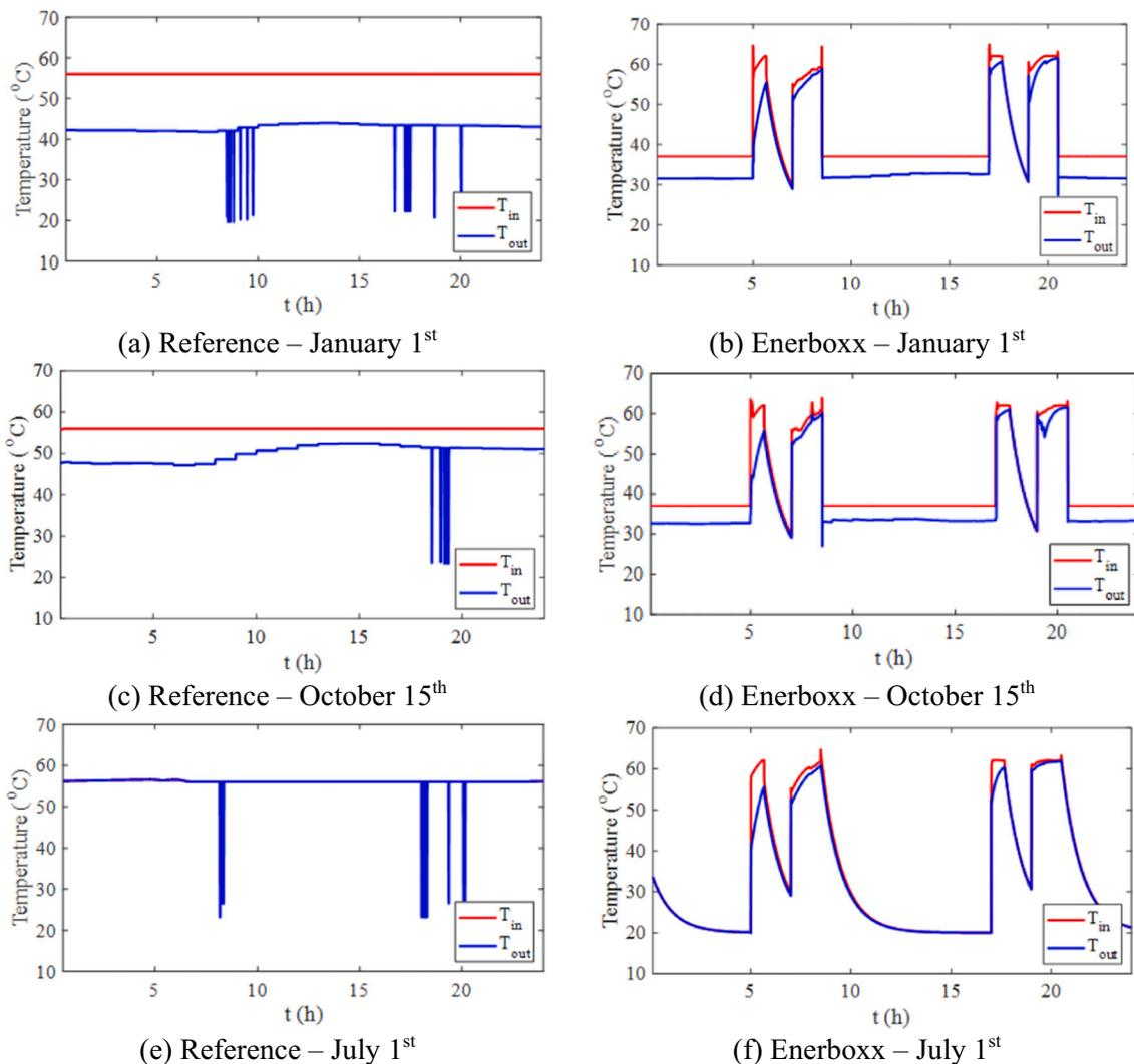
Fig. 12. Dwelling 1: Comparison of the reference and the enerboxx scenarios for different days during the year with the INTEMA tool.
