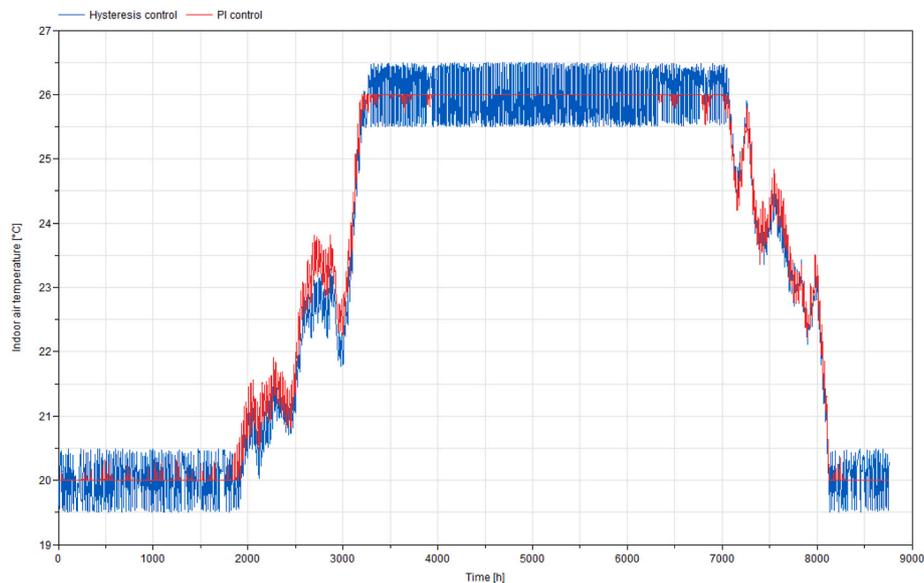
Fig. A2. Indoor air temperature distribution for the case with PI control and Hysteresis control (renovation case with reversible heat pump)
