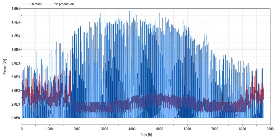
Fig. 12. Total electricity demand and PV production during the year for the renovation scenario.
