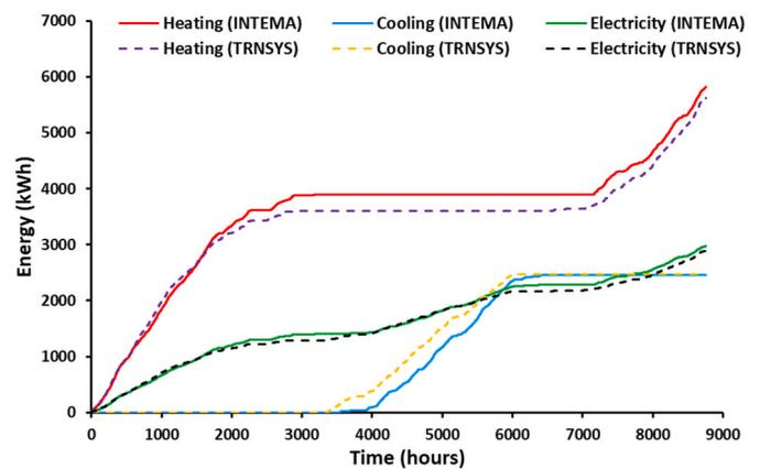
Fig. 3. Cumulative heating, cooling and electricity demands during the year with INTEMA.building and TRNSYS.
