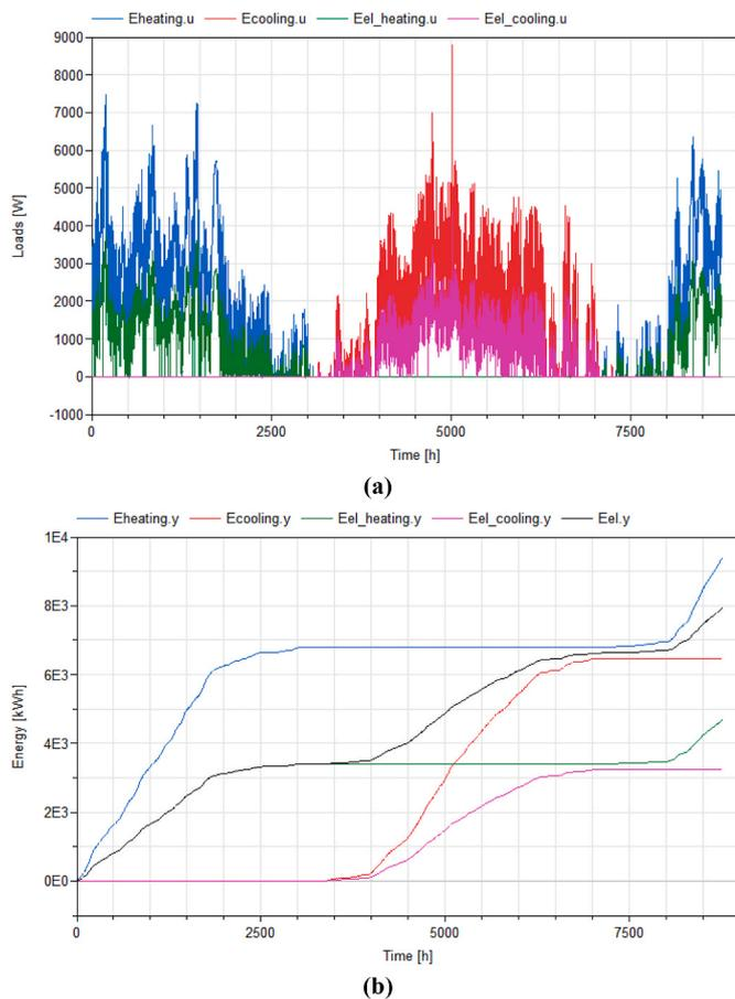
**Fig. 8.** Yearly heating and cooling demands of the B2 apartment (Heat pump for heating and cooling) for the baseline (a) Instantaneous loads and (b) Cumulative loads.
