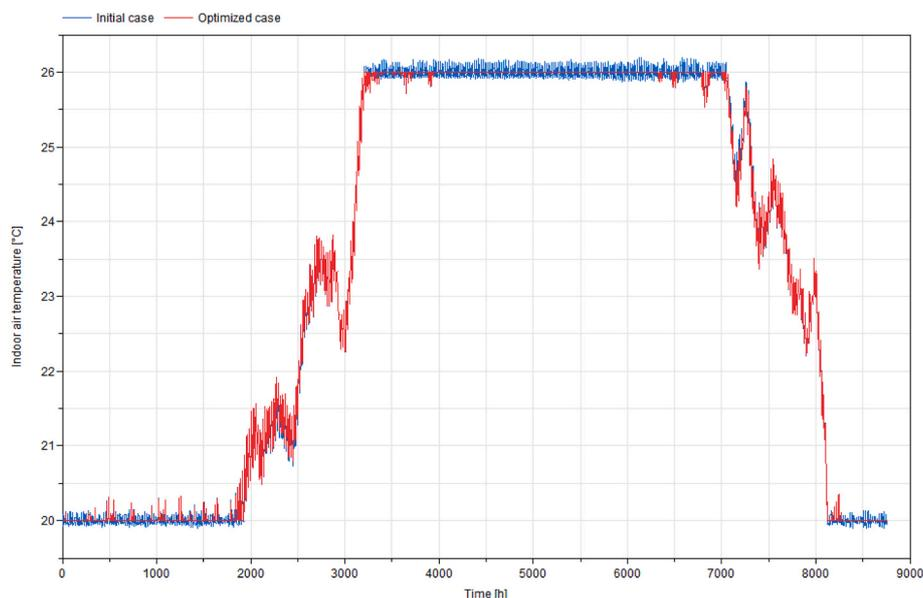
**Fig. A1.** Indoor air temperature distribution for the initial case without control tuning and for the optimized control tuning (PI control for the renovation case with reversible heat pump)
