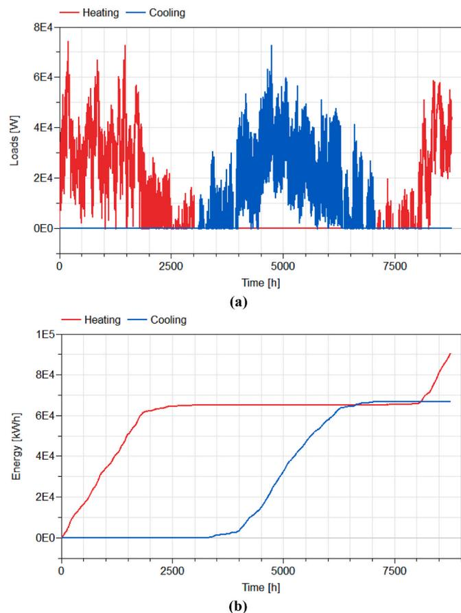
Fig. 6. Yearly heating and cooling demands of the building (8 apartments) for the baseline (a) Instantaneous loads and (b) Cumulative loads.
