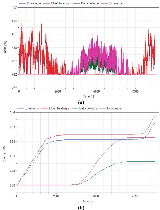
Fig. 7. Yearly heating and cooling demands of the B1 apartment (Natural Gas Boiler for heating and Heat pump for cooling) for the baseline (a) Instantaneous loads and (b) Cumulative loads.
