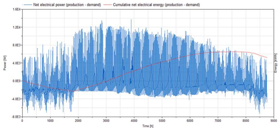
Fig. 13. Net electricity (production minus demand) of the examined building for the renovation scenario.
