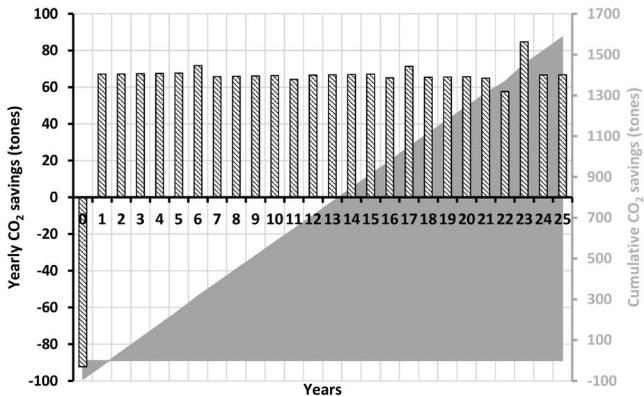
Fig. 16. Yearly and cumulative CO<sub>2</sub> savings for the renovation.
