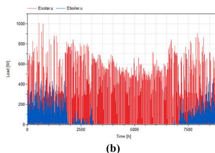
**Fig. 10.** (a) Yearly load variation for DHW of one apartment, (b) Boiler demand and solar useful production for the apartments (A1, B1, B3, A3).
