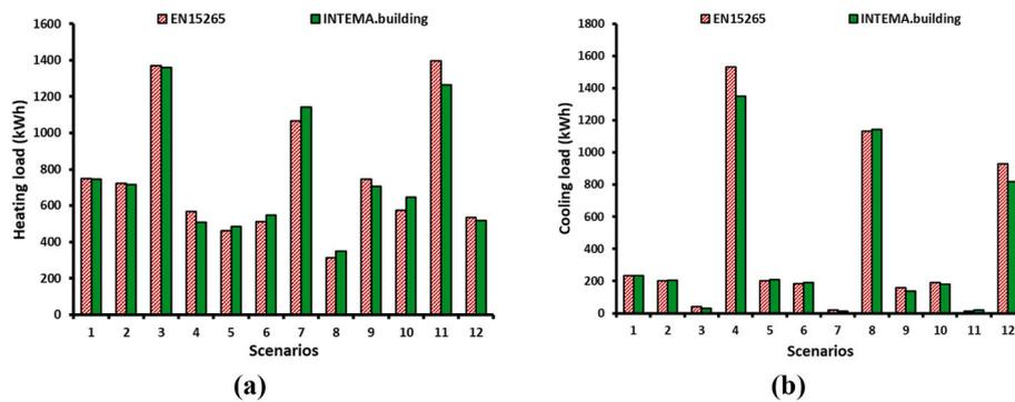
Fig. 2. Comparison of the simulation results with the EN15265 regarding (a) the heating loads, and (b) the cooling loads.
