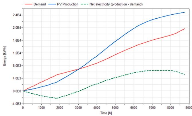
Fig. 14. Yearly variation of the cumulative electricity demand and PV production, as well as of their difference (Production minus demand) for the renovation scenario.
