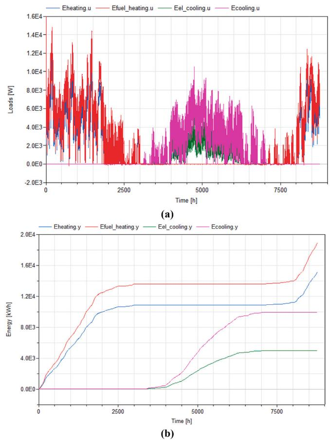
**Fig. 9.** Yearly heating and cooling demands of the B3 apartment (Oil Boiler for heating and Heat pump for cooling) for the baseline (a) Instantaneous loads and (b) Cumulative loads.
