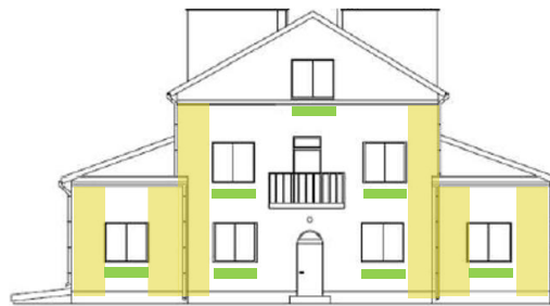
Figure 21 - Polish demo. Scenario 2. South facade. Positioning of vents (green) and PV panels (yellow)
