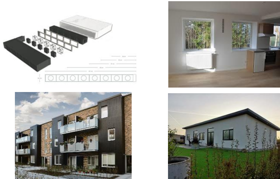
Figure 8 - MicroVent sustainable Ventilation system (InVentilate). Concept of the system (upper left) and examples of interior (upper right) and exterior architectural integration (below)
